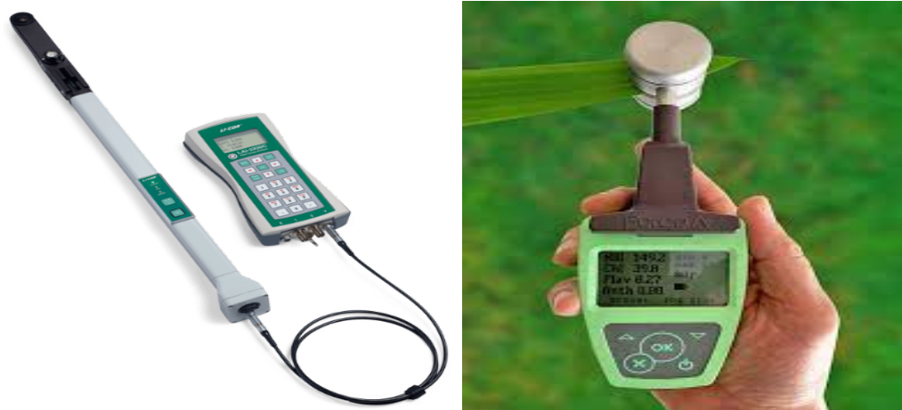
Figure 51. Instruments used for field campaigns. Respectively: on right, the LI-COR LAI2200c for LAI measurements and on left, the Dualex for chlorophyll content measurements.
